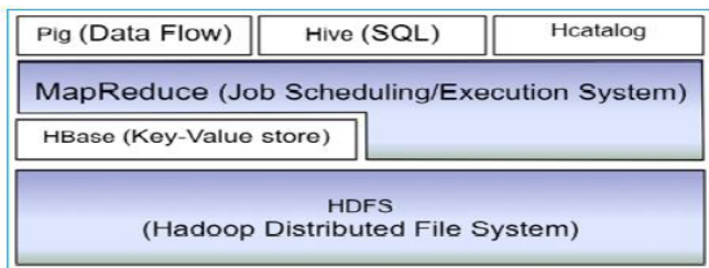
Fig 1: High Level Architecture of Hadoop
